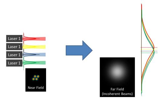
Figure 13: Principle of tiled aperture beam combining, showing far-field overlap of constituent beams
