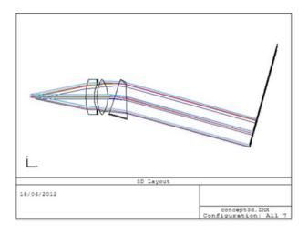
Figure 10: Optical design layout of prismatic wideband beam combiner demonstrator
