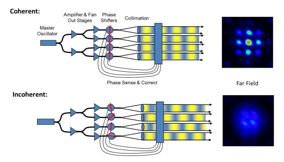
Figure 15: Typical derivation of phase-locked coherent beams in tiled aperture combining
