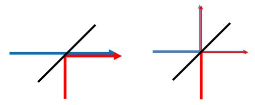
Figure 1: Elemental beam combining concept: ideal (left) and reality (right)
