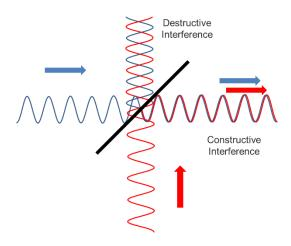
Figure 6: Efficient combining of two phase matched coherent beams
