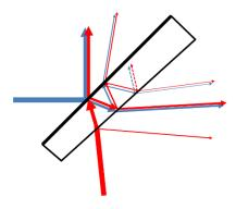
Figure 2: Multiple reflections in a beamsplitter substrate
