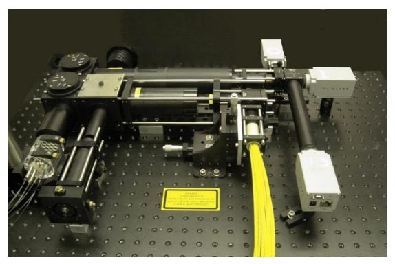
Figure 18: COTS realisation of the high power multi-channel coherent beam combining system
