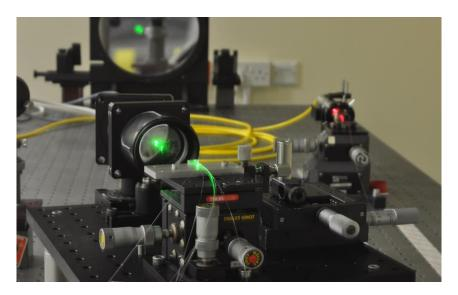
Figure 12: Prismatic beam combiner components during testing
