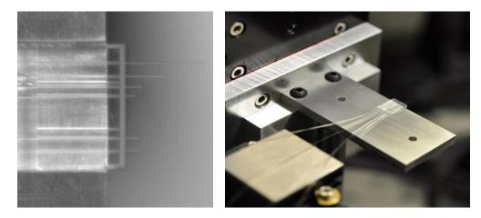
Figure 11: Detail of "V-groove" laser delivery fibre assembly
