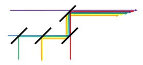
Figure 4: Multiple beam combination using Dichroic Mirrors
