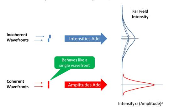
Figure 14: Difference between coherent and incoherent tiled aperture beam combining
