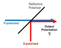
Figure 5: Twin beam combining using a reflective polarizer
