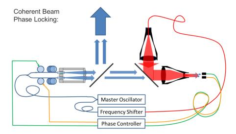
Figure 17: Interferometric method of producing phase-locked coherent beams
