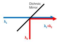
Figure 3: Twin beam combination using a Dichroic Mirror
