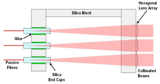
Figure 16: Pure Silica monoblock lens assembly for multiple high power beam alignment
