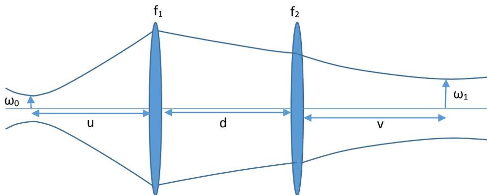
Figure 2 Beam waist formation by a pair of lenses.
