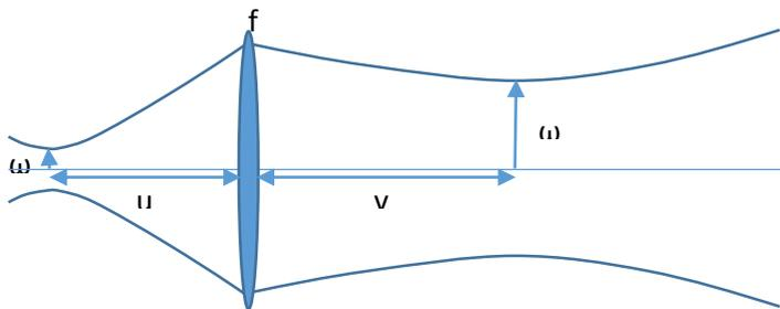
Figure 1 Beam waist formation by a single thin lens.
